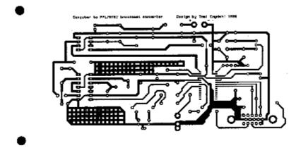
You can print out the picture at correct resolution to a laser printer (6.83x3.87 inches) to a slide and propaly use it as a mask for making a circuit board of your own. If you have a postscript printer or a suitable viewer/printing program you can download zipped Postscript version of the circuit board which automatically prints to right size.
